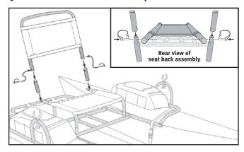
Slide the seat stubs onto each end of the seat back frame. Next, slide the seat back panel onto the seat back frame. Then place the assembled seat back into position on the outsides of the seat frame and secure to the seat base with the two long clevis frame pins.
